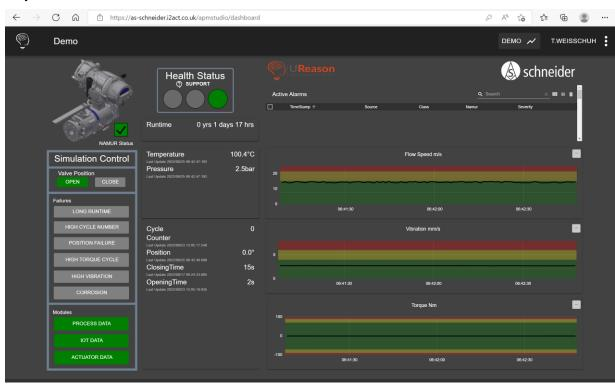
**Picture 1:** With the Digital Valve Kit, users can permanently check their valves via software to ensure that they are working properly.
