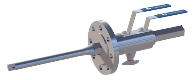
**Picture 4:** The customized injection quill consists of two shut-off valves and one bleed valve.
